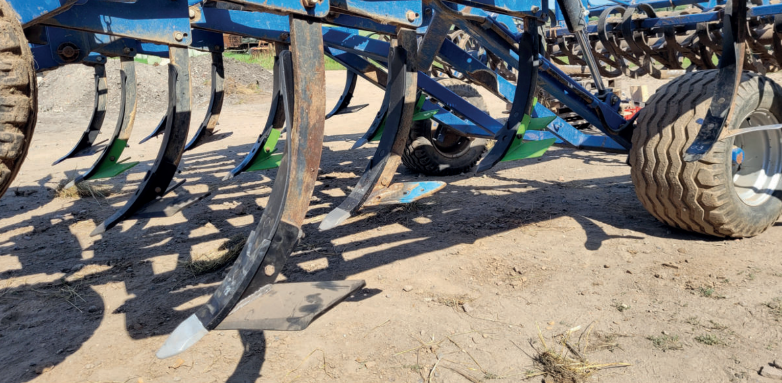
Figure 3: Field trial with modified cultivator points
