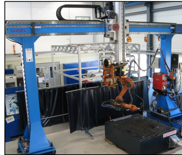
Portal with KR 15 and MIG/MAG-welding appliance
