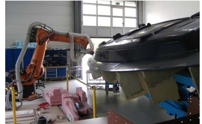
Robot milling of large components in connection with flexible component holder
