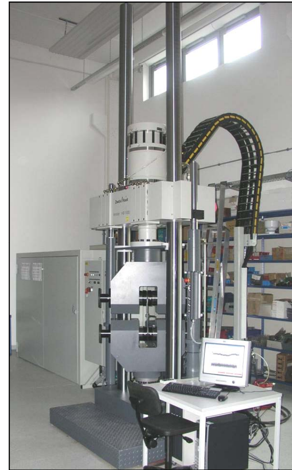
Servo-hydraulic tester HB 1000 at fatigue tests of mechanically joined connection samples in the Fh AGP-Laboratory
