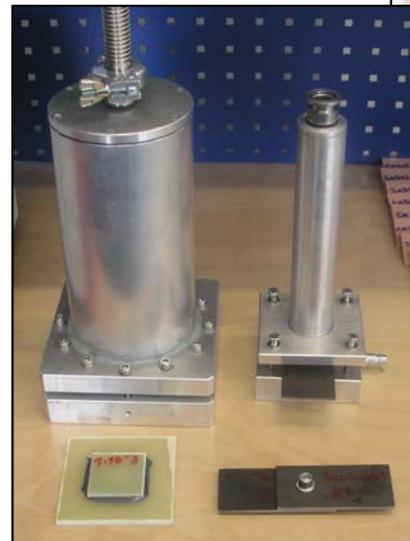
Vacuum/excess pressure cylinder for measuring tightness of adhesion and mechanically joined connection samples in connection with the helium leakage test device
