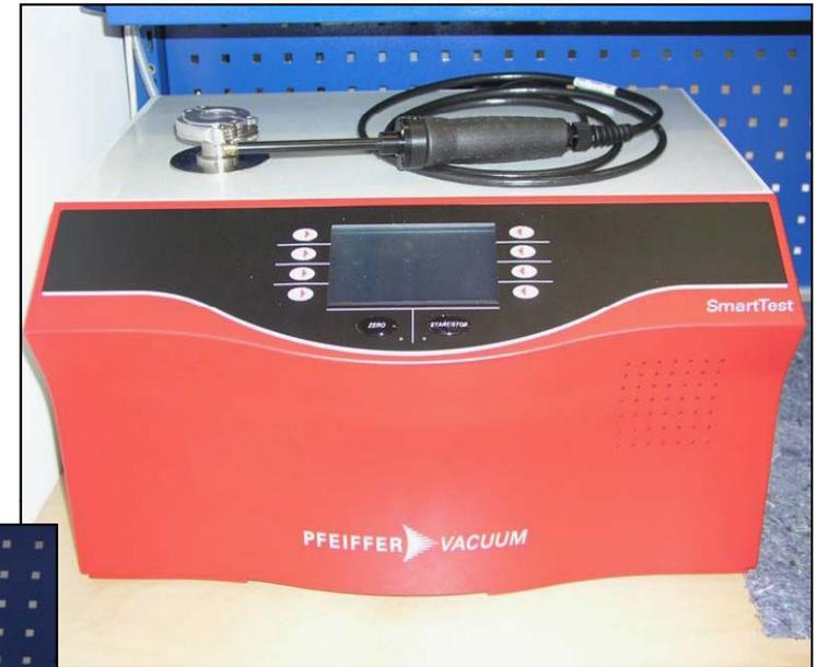
Helium leakage test device HLT 160/560 with sniffing sensor for leakage search
