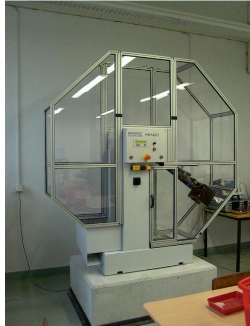
View of the impact testing machine PSd 450
