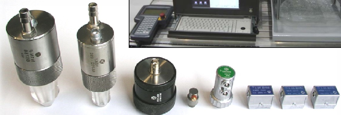
Ultrasonic- probes for diverse materials and testing tasks
