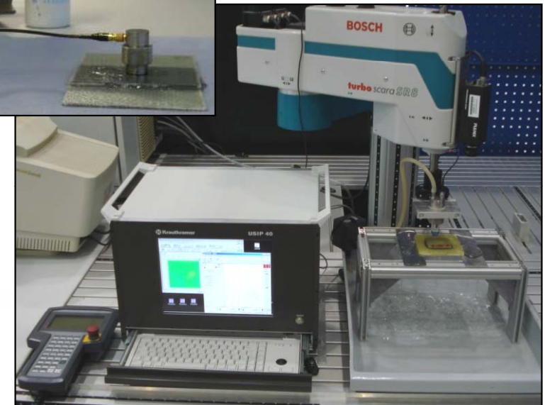
Automated US-test station with water jet coupling for the exposure of C- images
