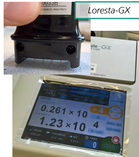
Measuring the specific electrical conductivity of a metallic coating
