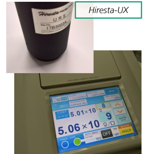
Determination of the specific surface resistivity of a ceramic sample
