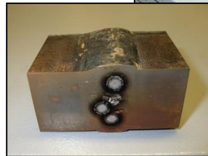
Analysis of welding deposit with test replica
