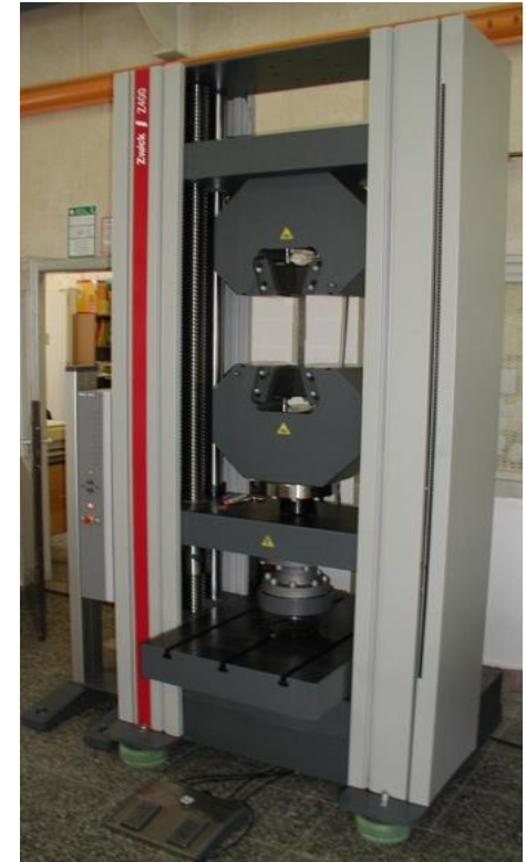
View of tester Z400E during tension test of blind riveted flat shear tension
