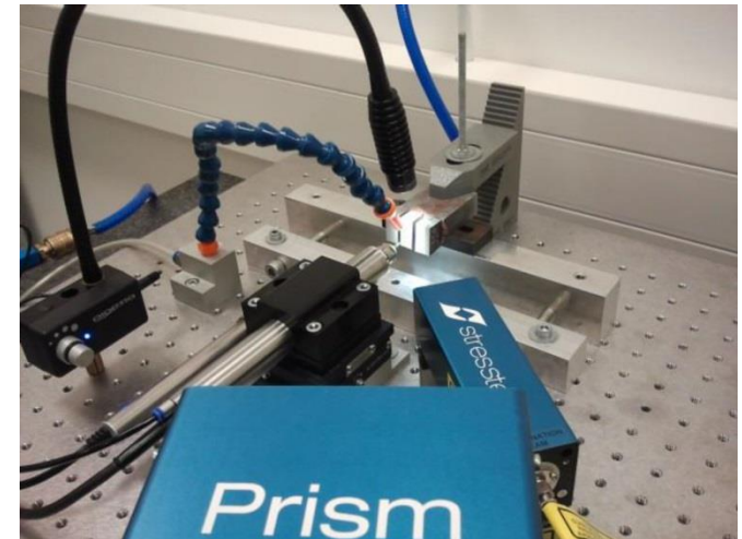
Measuring setup to determine the state of internal stress in thermally sprayed samples. Analysis system consisting of a laser light source, lighting stand, camera unit and electrical high-speed drilling machine
